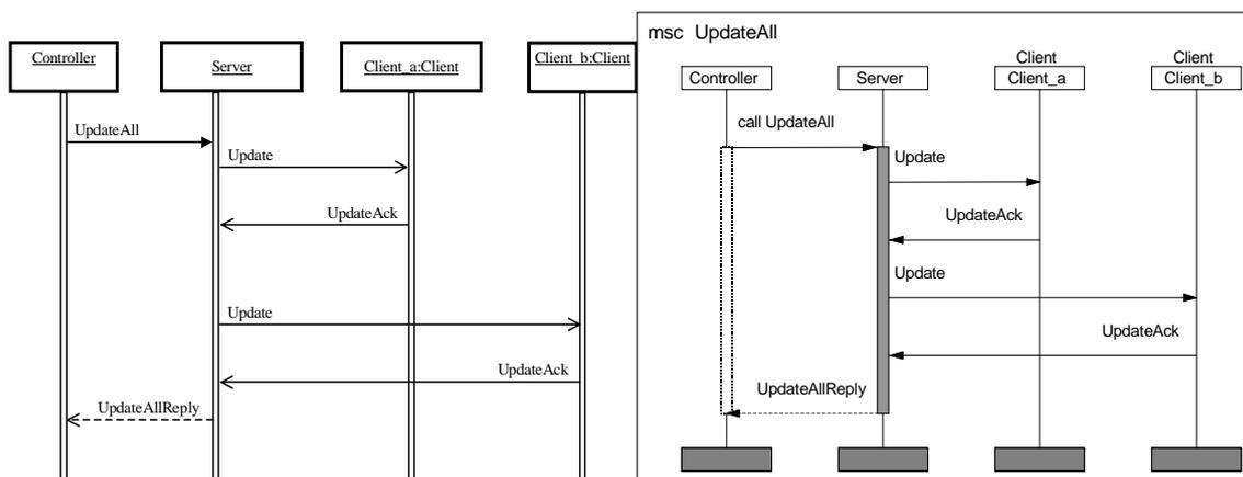
Figure 96: UML sequence diagram and corresponding MSC
