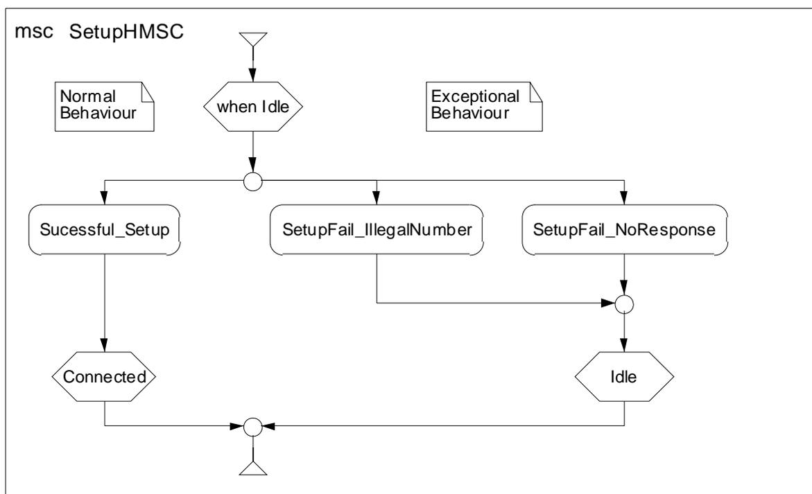
**Figure 2: Example HSMC**
