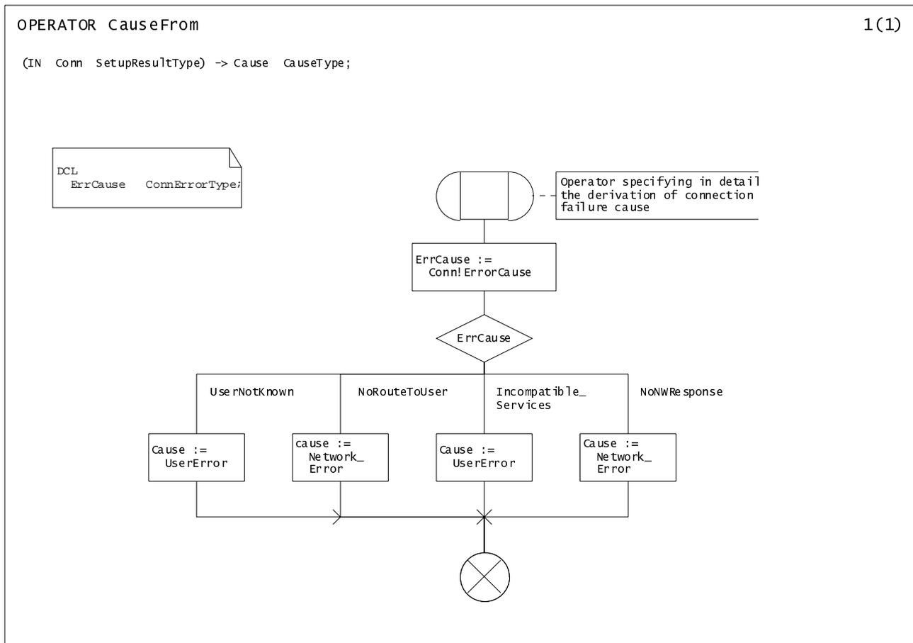
Figure 34: Example of detailed operator diagram
