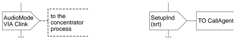
Figure 66: Examples of the use of TO and VIA
