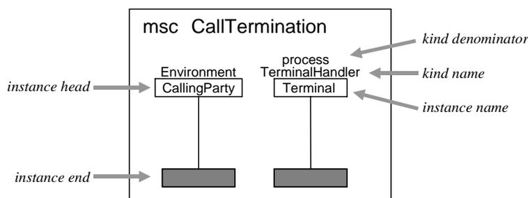
Figure 77: Placement of instance name and kind name
