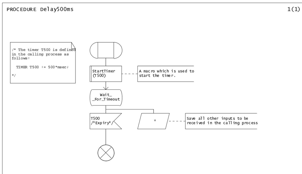
**Figure 27: Example of a procedure containing a state**
