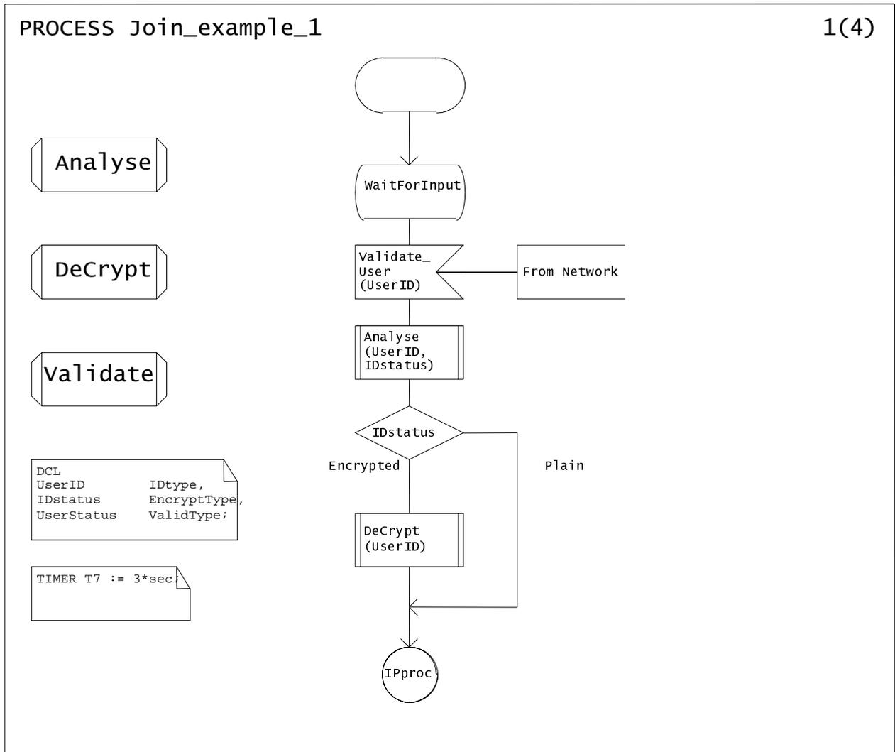
Figure 9: Paging using a connector symbol (page 1)
