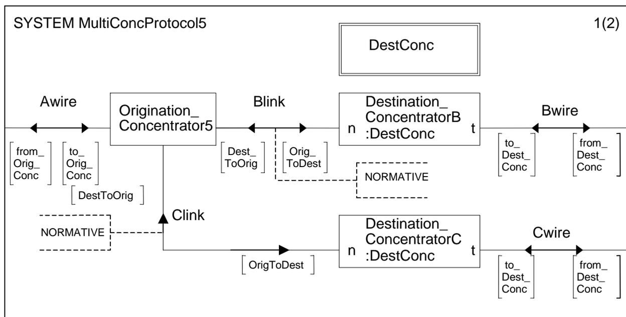
Figure 55: Static SDL model for a multi-link scenario
