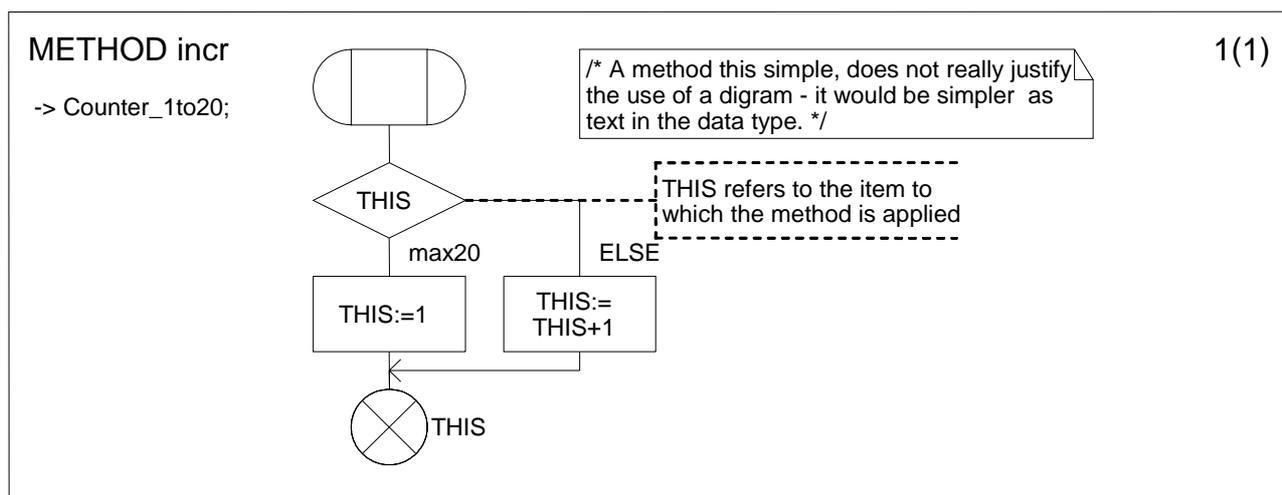
**Figure 30: Method diagram**
