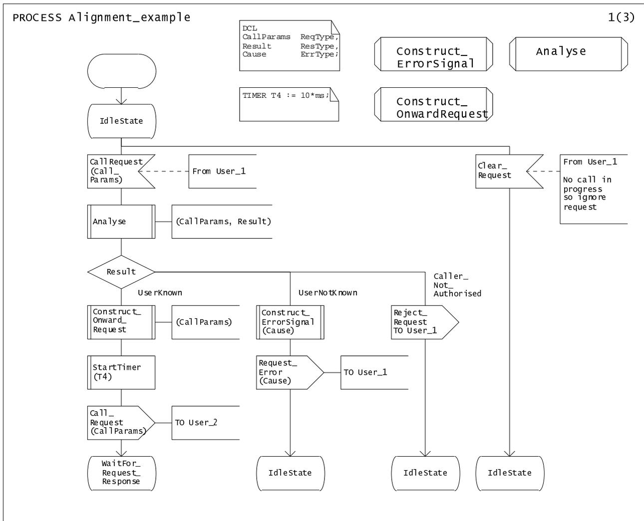
Figure 8: Transitions aligned on a single page
