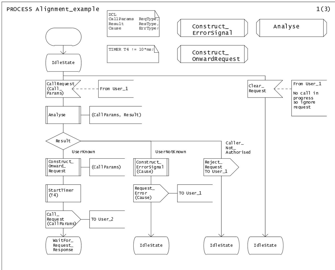
Figure 15: Example showing the alignment of NEXTSTATE symbols
