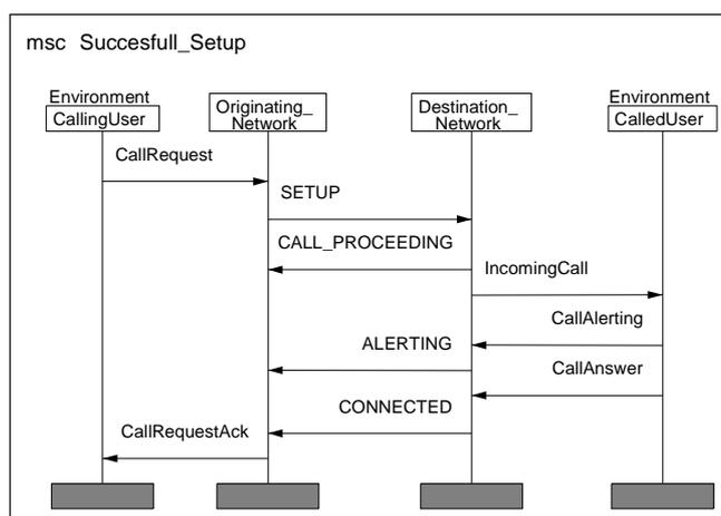
Figure 79: MSC with instances representing the environment
