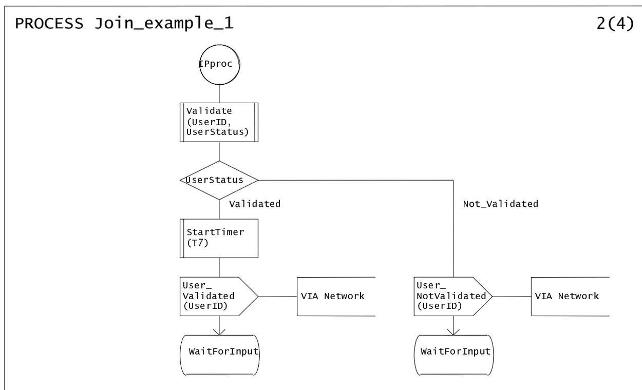
Figure 10: Paging using a connector symbol (page 2)
