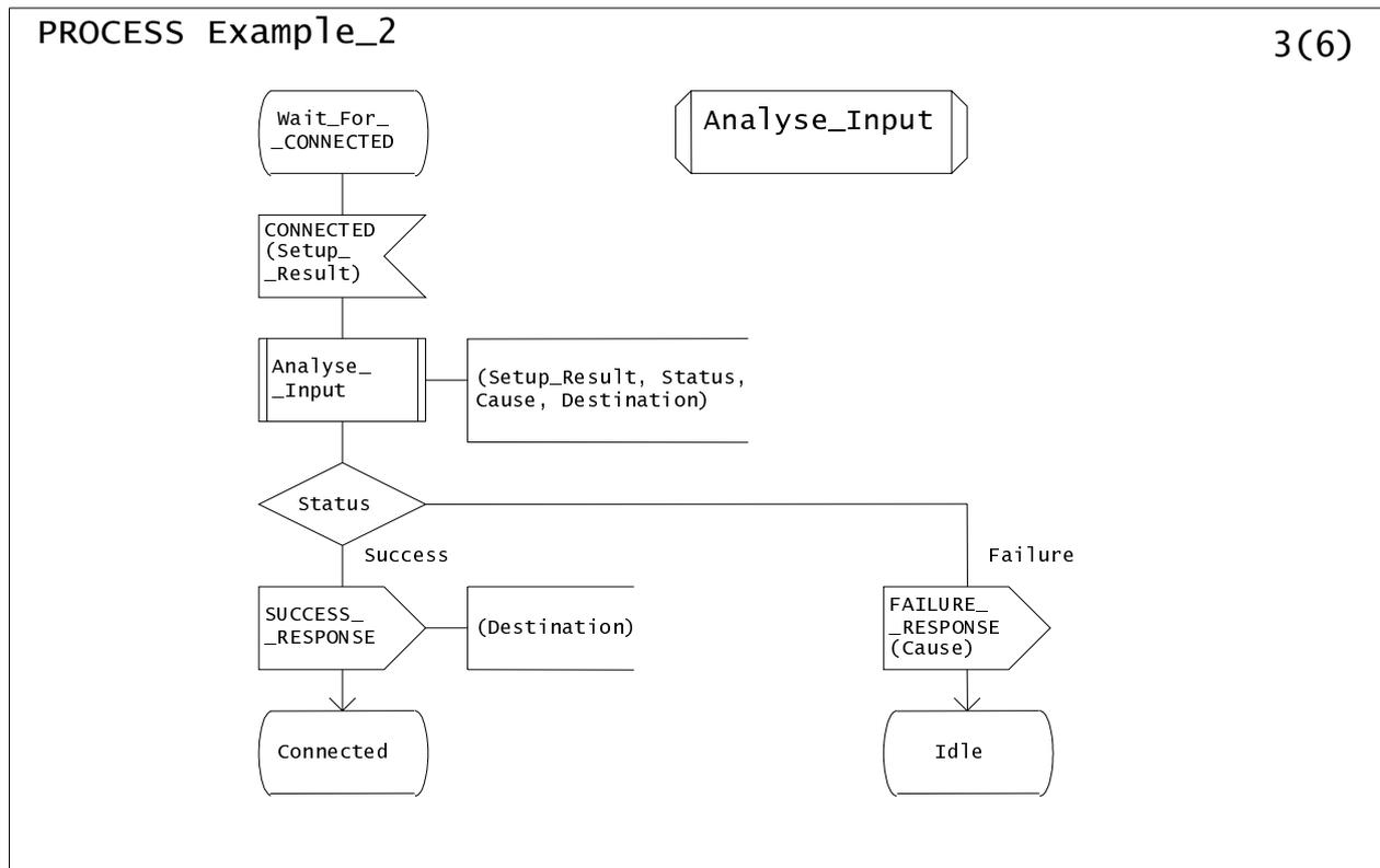
Figure 20: Message analysis example using a procedure
