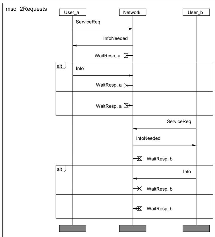
Figure 90: Separated timer symbols and timer identifier
