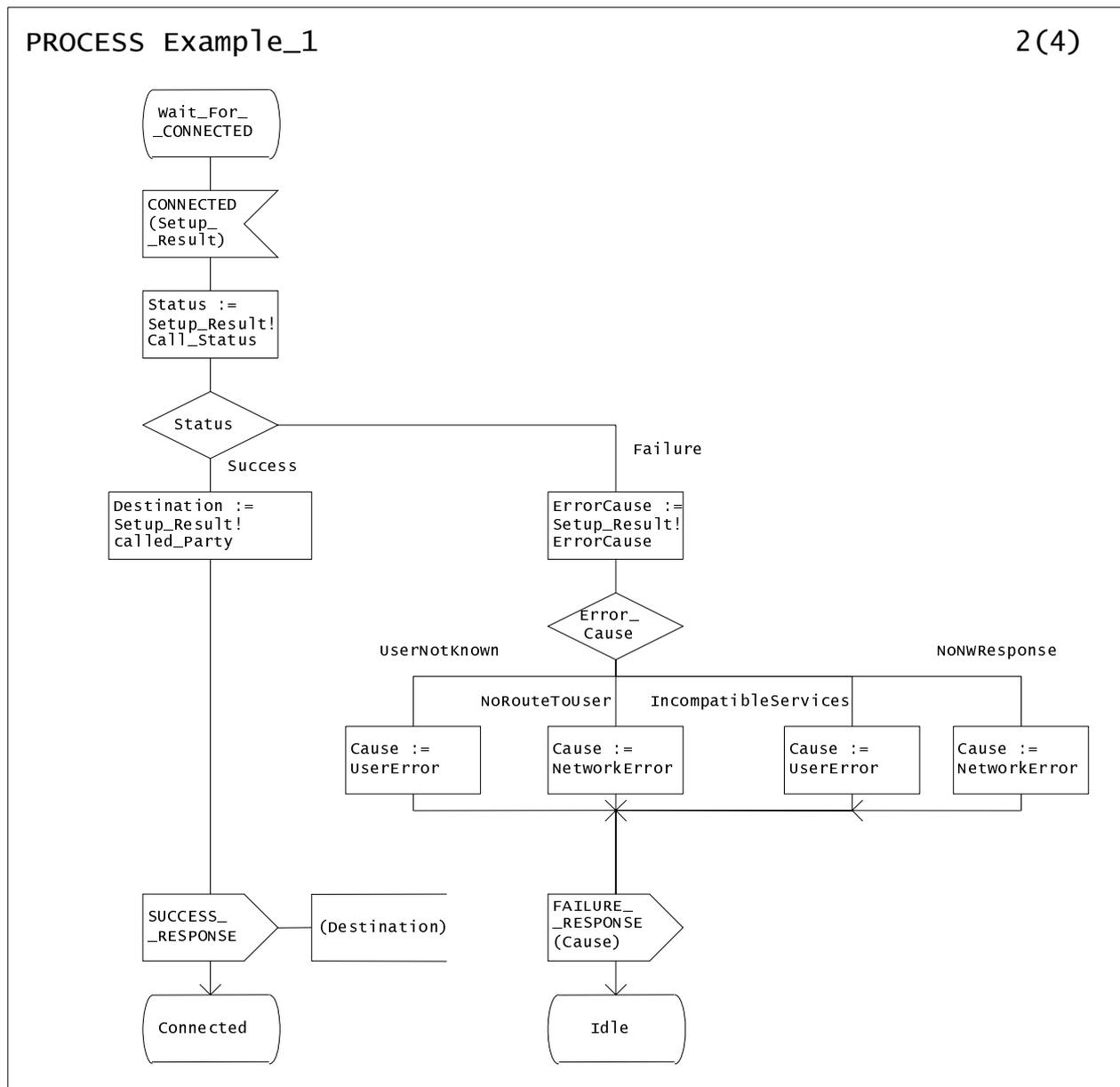
Figure 19: Message analysis example without the use of a procedure
